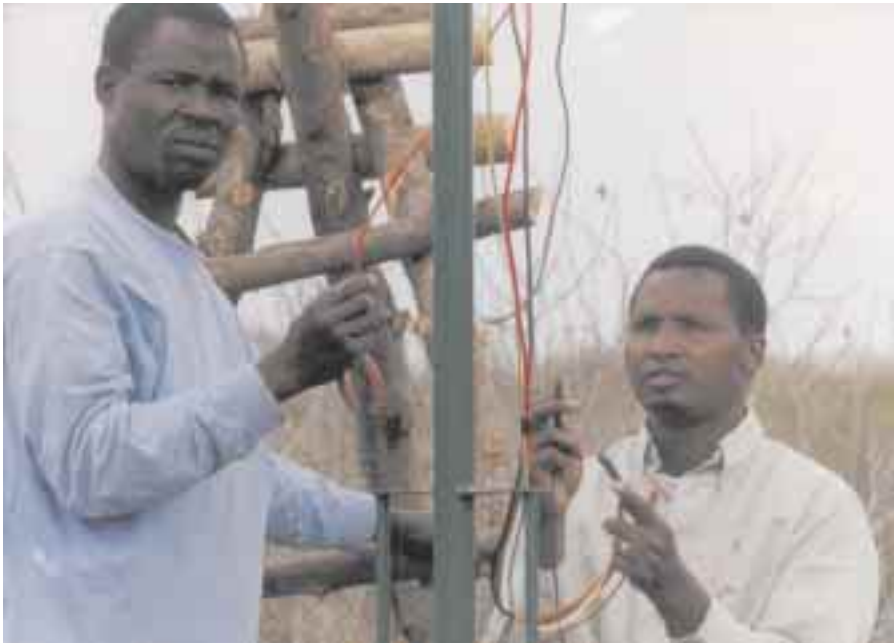
Students David Omgacho and Peter M. Ngalu from CWMS check array voltage.
